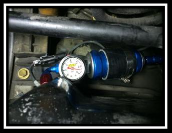
The new clamp goes through the factory bracket for the factory fuel filter. The original filter is much larger in diameter, so a new smaller SS hose clamp is required.
