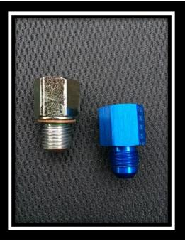
The pictures above show the original hard line adaptor fitting and the Earl's -6AN adaptor. The original Porsche fitting's threads are too long and must be cut down .20" in order to not bottom out in the Earl's piece. The Earl's piece is a 14 X 1.5 mm to -6AN adaptor fitting part number 9894DBH. I used a new copper crush washer.
