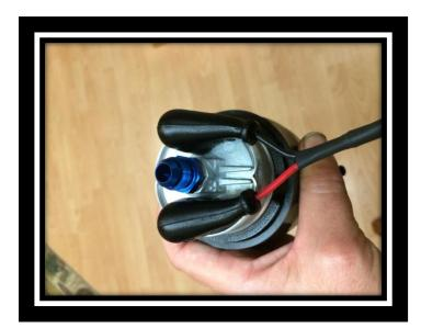
Note: The picture above shows the connection before I knew how loud the pump was without the factory coozie. Do not use the above isolation method for mounting your fuel pump!
