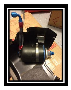
The final picture above shows the final version with the factory coozie installed and mounted to the fuel pump cover. Follow the many online procedures for making the actual AN flex line connections. I used the proper Earl's lube but I am sure any light weight oil would be fine. Either place electrical tape on your adjustable wrench or buy the correct aluminum AN wrenches or you will mar your pretty fittings. See some pictures below:
